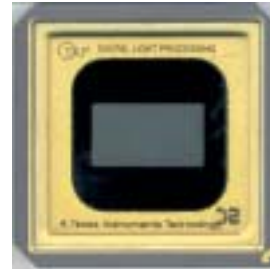
DMD array consisting of microscopic mirrors.
