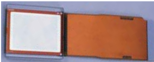
The D-ILA device from JVC, with a resolution of 2048 x 1536 pixels and a 1.3-inch diagonal.
